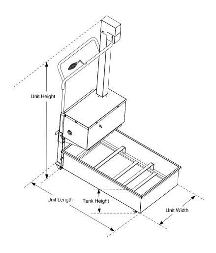
YPF95 Series filter unit dimensions (unit and tank heights are measured from bottom of casters to top of unit and tank, respectively).
